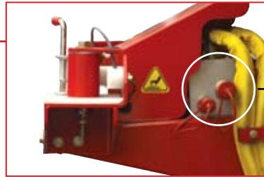
Location of hydraulic manifold (MH-400).
